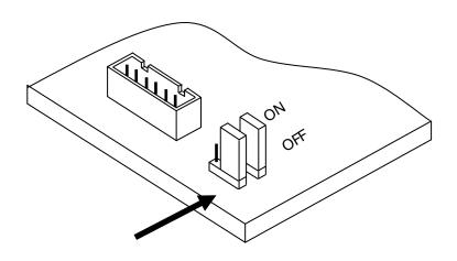
Move the mini jumpers to the **ON** position **BEFORE** going off-hook.
