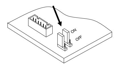
When programming is completed, move the mini jumpers to the **OFF** position.
