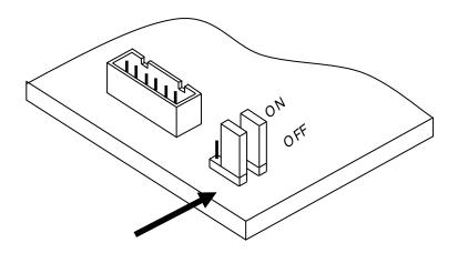
Move the mini jumpers to the **ON** position BEFORE going off-hook.
